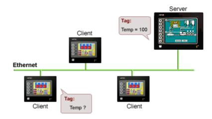
The G3's OPC link is an easy way to connect multiple G3s together. G3 to G3 communication is achieved in minutes using direct tag access from one unit to another.
