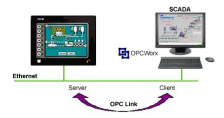
Red Lion's OPCWorx is a configuration tool for our OPC servers. This easy-to-use software tool allows you to create and configure an OPC server to communicate with the G3 series HMI, the Data Station Plus or the Enhanced Master, as well as any device that supports Modbus.
