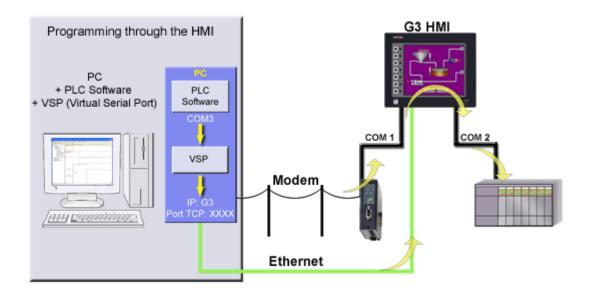
Pass-through programming is a unique feature which allows you to program your connected devices remotely\*. Using either a modem or an Ethernet connection, you can reprogram your PLC, motor drive, etc. from anywhere in the world.
