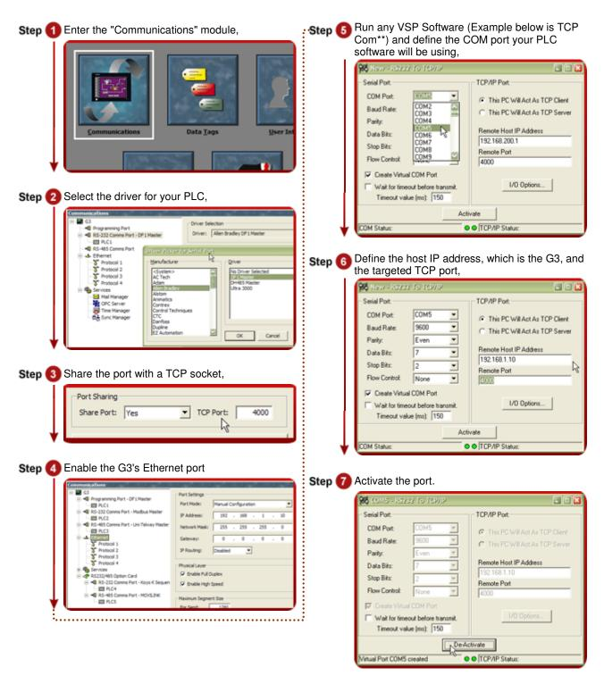
Your PLC software is now ready to use this virtual port as if it was connected directly to the PLC.
